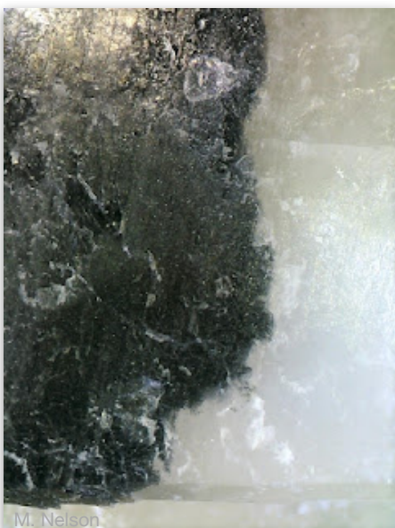
Above: Photomicrograph of boundary of klockmannite and calcite (specimen above). Photo: M. Nelson
