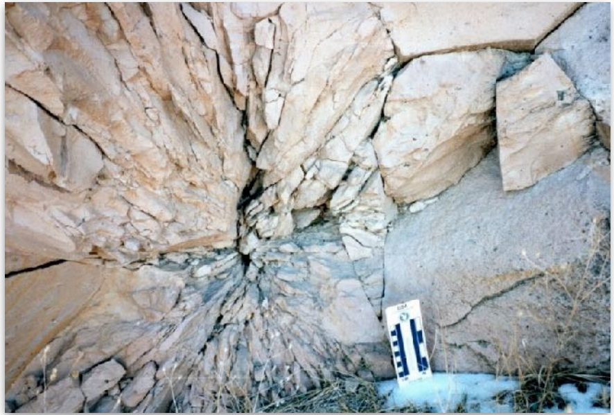
Fig 10: Fracture pattern in the Castle Rock Rhyolite from a blast during quarrying at the Madge quarry. Photo date 1995 by S. W. Veatch.
