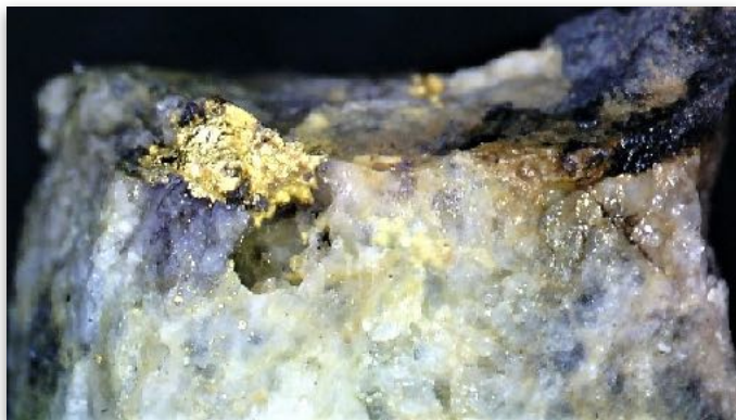
Above: "Sponge" gold of roasted ore from the Ajax Mine. Width FOV ~7 mm. Photo: From the former collection of CSMS member Willard Wulff and mounted 1985.
