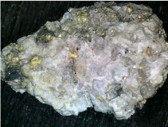
Above: Gold in roasted ore from the El Paso Mine at Cripple Creek. Width FOV ~1.95 cm. Photo: Originally in the collection of CSMS member Chris Christensen and then acquired by CSMS member Willard Wulff.
