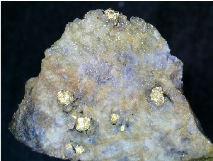
Above: Blister and "sponge" gold of roasted ore from the Ajax Mine. Width FOV ~1.1 cm. Photo: From the former collection of CSMS member Willard Wulff and mounted 1985.
