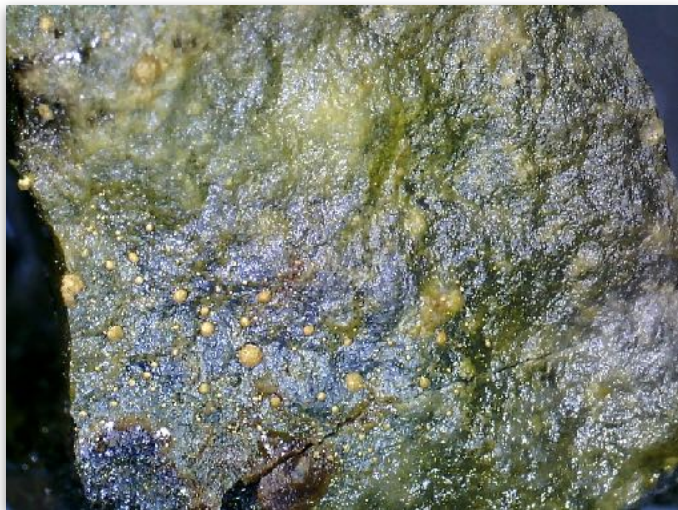
Above: Blister of roasted gold ore from the Ajax Mine at Cripple Creek/Victor. The underground mine is no longer in operation and may be, or is, consumed by the large open pit known as the Cresson Mine. Width FOV ~9 mm.
