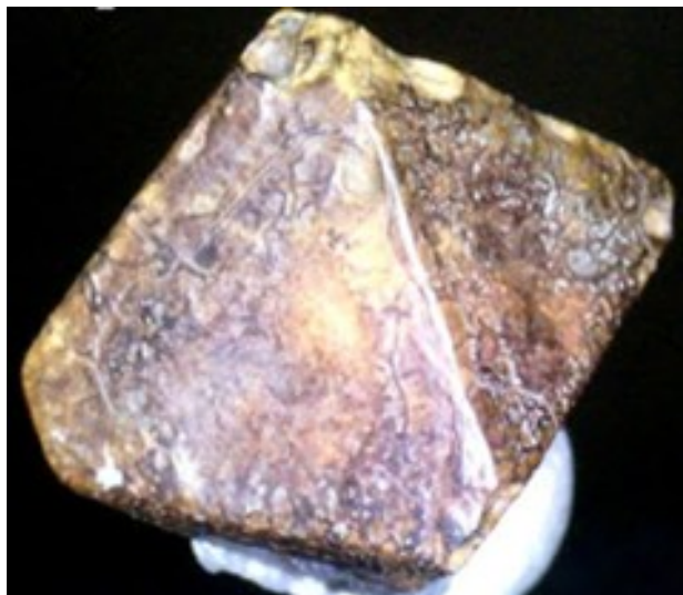
Fig. 3. Octahedron of limonite pseudomorph after pyrite. Axes are ~1.2 cm.
