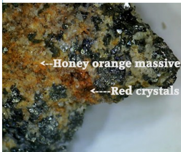
Fig. 1. Photomicrographs of greenockite occurring as honey orange encrustations with a couple of red poorly formed crystals. Width ~1.1 cm. Dark metallic mineral is most likely arsenopyrite.
