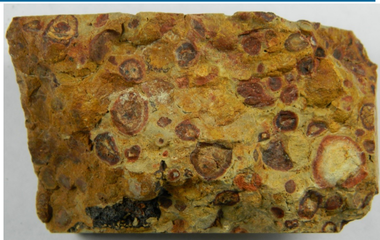
Fig. 1. Pisolitic bauxite from Pulaski County, Arkansas, collected late 1960's. Width ~6.5 cm.
