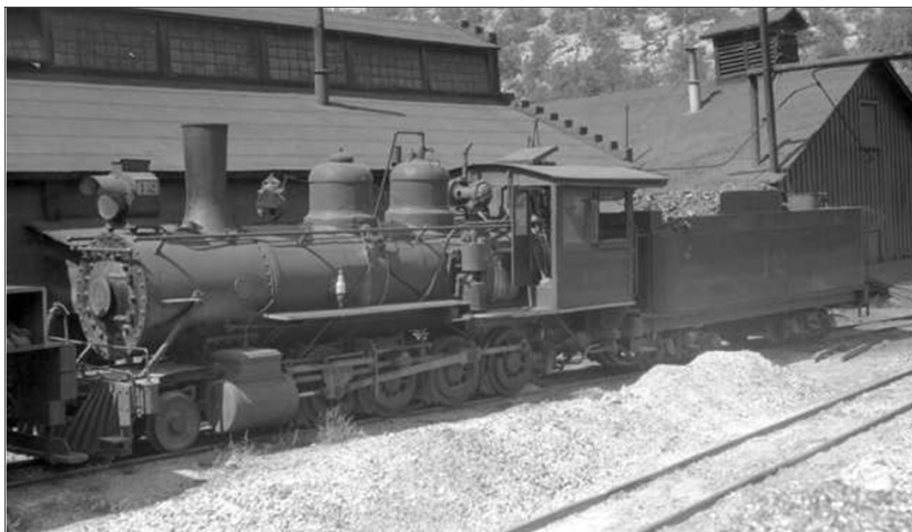
Fig. 5. 2-8-0 #12 engine built by Baldwin in March 1896 for the Florence & Cripple Creek RR. It was bought by the Uintah in 1917. Courtesy of photographer Otto Perry and The Uintah Railway.
