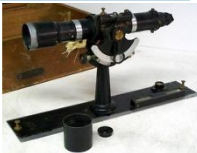
Fig. 11. I used a Gurley alidade where the geologist looked “down” into the eyepiece rather than “straight ahead” toward the stick. Angles were measured and trigonometry tables allowed the geologist to determine elevation (plus or minus from the station) and distance. Distance to the stick was drawn along the ruler/base. Photo from sale items on EBAY.
