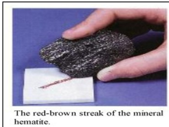
Fig. 2. Determining the streak of a mineral. Photo courtesy of California State University, Pomona.
